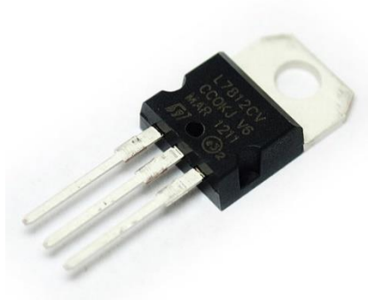
Gambar 2.9 Regulator Tegangan (Sumber: Boylestad, 2007)
